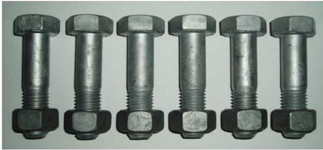
a.) bolts before test
