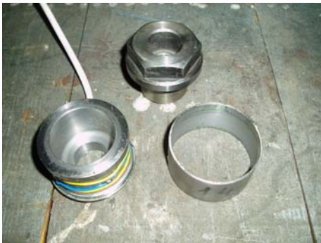
Fig. E3 Parts of a load cell (nut, measurement part, stovepipe).
