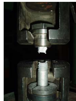
Fig. B66 Bolt failure.
