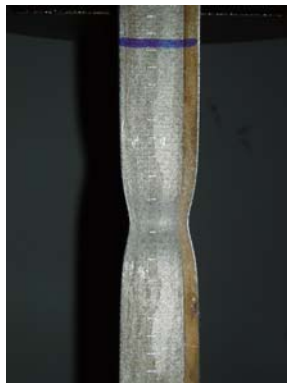
Fig. B48 Test specimen failure 1 (B3).
