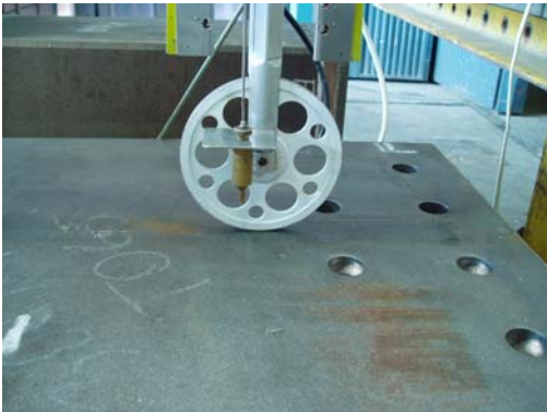
Fig. D3 Measuring wheel with inductive transducer.
