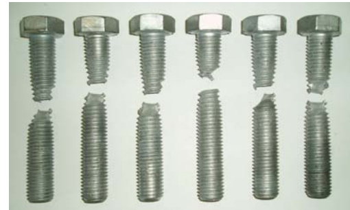
b.) bolts after test
