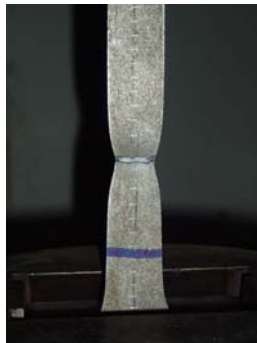
Fig. B26 Test specimen failure 2.
