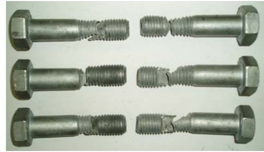
b.) bolts after test
